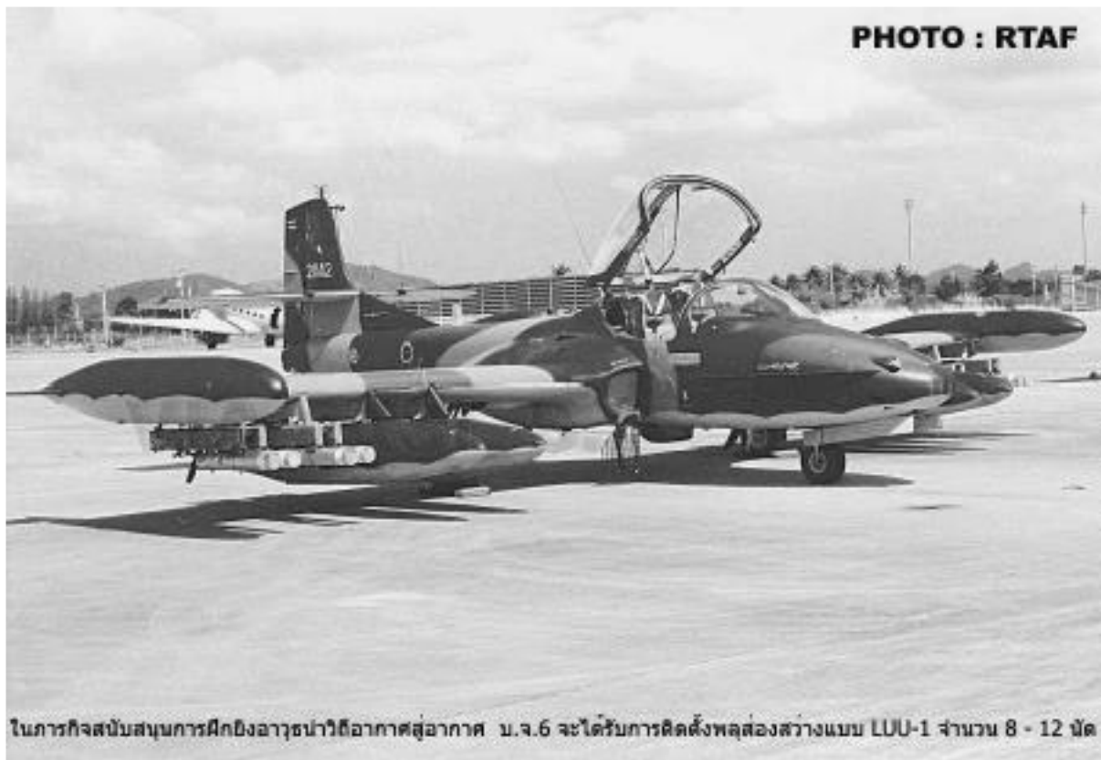
In the mission to support air-to-air weapons training, the A-37B was fitted with launchers for 8-12 LUU-1 flares. D Wing 21), and SQNLDR Phiphop Buawirat.
