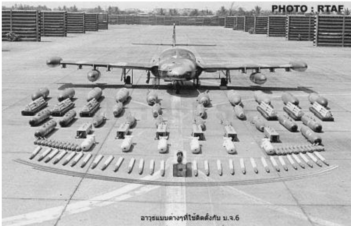
The range of ordnance which can be carried by the Attack Type 6 (Dragonfly) aircraft.
